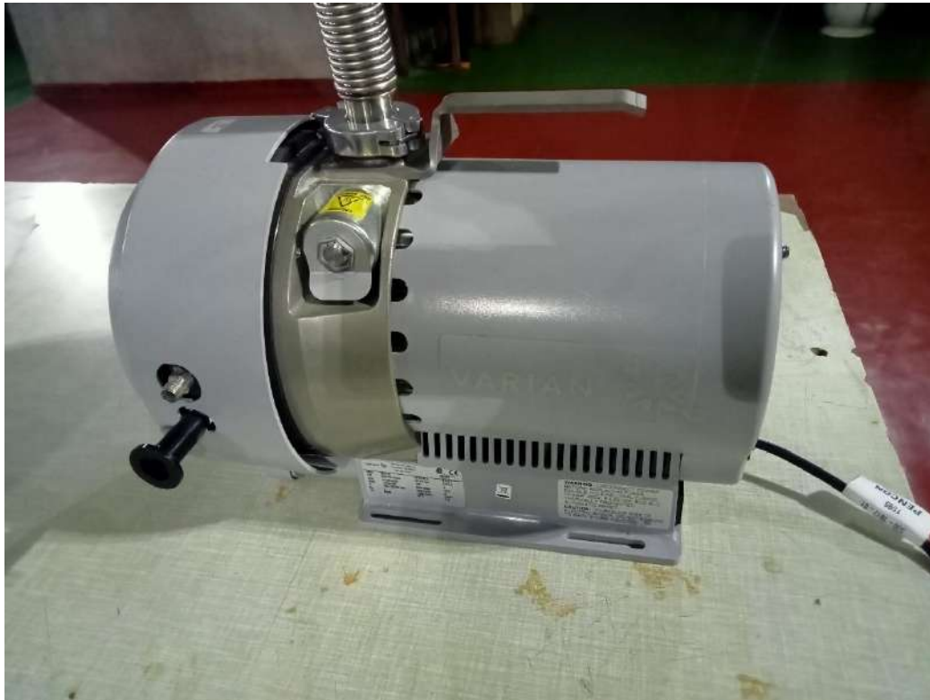
Evacuation pump of CCD camera
